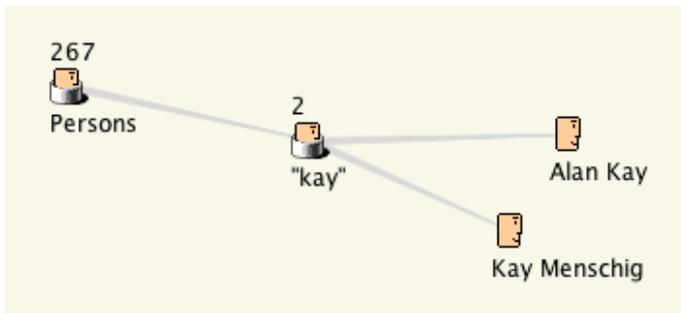
**Fig 5:** In DeepaMehta large amounts of data are displayed as a ton. A ton represents a query to the corporate memory and the result set at the same time. In this example an unspecific person search results in 267 topics — too much to reveal at once. Applying a filter “kay” yields to a result set small enough to be revealed immediately.
