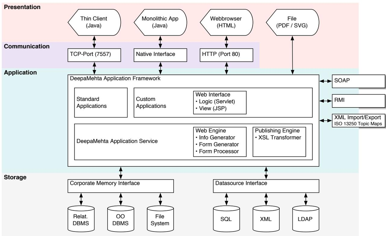
**Fig. 6:** DeepaMehta is a multi-layered distributed software architecture. The heart of the DeepaMehta software architecture consists of an application server. DeepaMehta applications are developed in the scope of the DeepaMehta application framework and run at server-side. Applications can access a variety of data sources and can be served to a variety of frontends.
